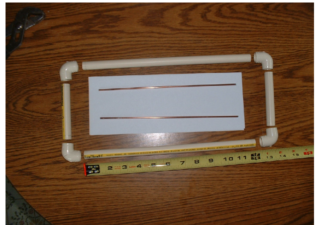
1/2" PVC, elbows, and welding rod
